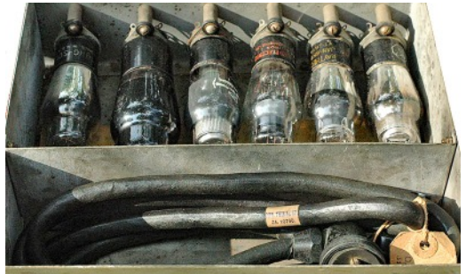
Spare valves and mains/battery leads were stored in the drawer above the receiver.
