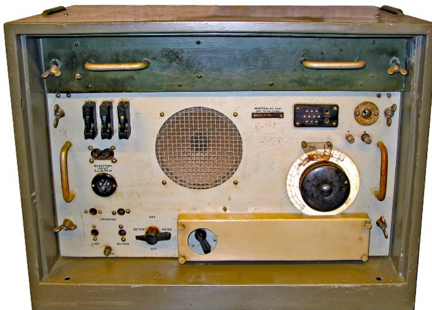
Reception Set R208 manufactured by Radio Gramophone Development Co. (RGD) with serial number 3068. A coax socket was fitted in addition to the (repositioned) aerial and earth terminals. Note the rarely encountered cover fitted over the control knobs allowing access to the volume control only.
